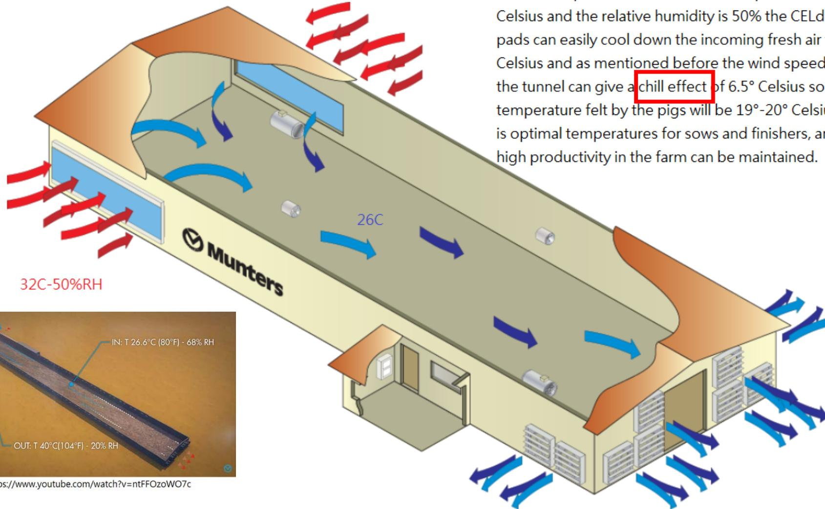
As an example, when the outdoor temperature is 32° Celsius and the relative humidity is 50% the CELdek® pads can easily cool down the incoming fresh air to 26° Celsius and as mentioned before the wind speed from the tunnel can give a chill effect of 6.5° Celsius so the temperature felt by the pigs will be 19°-20° Celsius. This is optimal temperatures for sows and finishers, and the high productivity in the farm can be maintained.
